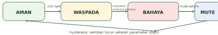
Gambar 5. State machine kendali alarm bertingkat
